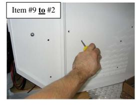
Loosely bolt **Passenger-side Bench/Wall** assembly to 3<sup>rd</sup> **Compartment Bulkhead** using ½" x ¾" Carriage bolts and serrated nuts
